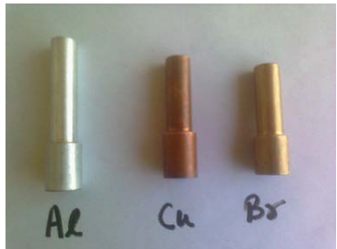
Fig. 1: Aluminum ,Brass, copper Electrodes of 15mm diameter
